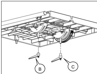
• Get assistance to slide table assembly so that the saw blade passes through the slot of table. When the saw blade reaches the rectangular hole in the center of the table, rotate the table assembly by 90 degrees according to the arrow.
