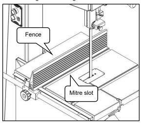
The aluminum fence plate can be installed in one of two positions; vertically or horizontally as shown in the following figure. Horizontal position is useful for smaller workpieces.
