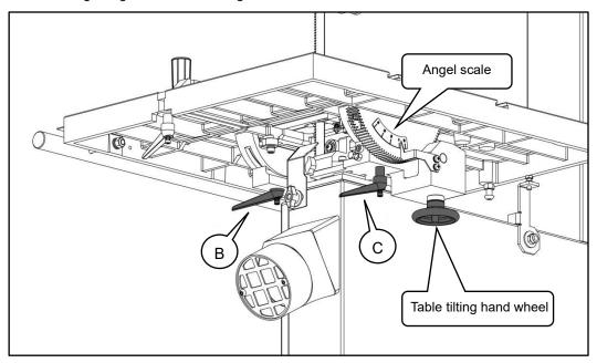
• The table has three preset angle positions, Use an angle gauge to check the accuracy of the preset angle positions and adjust the angle stop if necessary.
