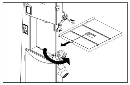
Pass the angle locking screws to the holes on the table tilting base, attach the table assembly to the tilting base, and secure the table by replacing the short locking handle B and long locking handle C.
